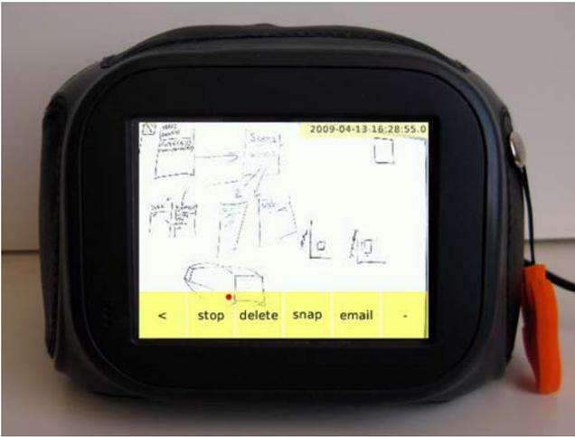
Figure 6: The ReBoard persistent user interface running on a Chumby device. The interface provides one-touch manual capture and a persistent display of content archived by the ReBoard system.
